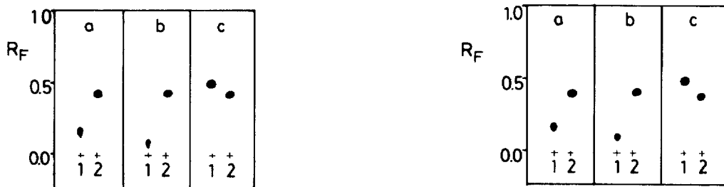
Fig. 2. Effect of pH of the stationary phase on the TLC behaviour of dabsyl morphine and dabsylamide in chloroform—absolute ethanol (30:2). (a) Silica gel 60 F_{254} ; (b) silica gel 60 F_{254} exposed to acetic acid vapour; (c) silica gel 60 F_{254} exposed to ammonia vapour. Samples: (1) dabsyl morphine; (2) dabsylamide.
